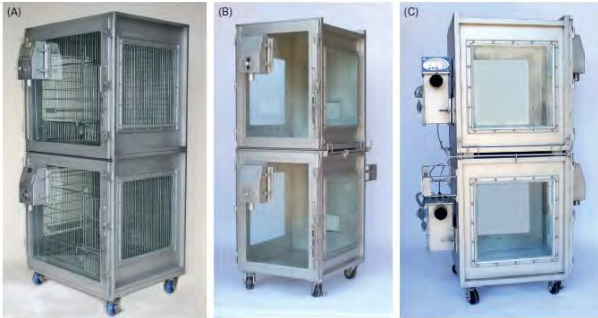
FIGURE 27.1 The primary containment cage shown is designed to house nonhuman primates. The clear Lexan® panels allow plentiful light penetration and a HEPA filtered air inlet box in the front of the cage (A) has a connection for a controlled warming system for animals recovering from anesthesia, or that otherwise become hypothermic. Cages are easily removed for cleaning the interior of the primary containment envelope (B). The blower motors and HEPA-filtered exhaust boxes are located on the back of each cage (C). Photos provided courtesy of Carter Systems, Inc.
