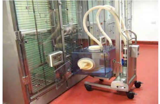
FIGURE 27.1 The primary containment cage shown is designed to house nonhuman primates. The clear Lexan® panels allow plentiful light penetration and a HEPA filtered air inlet box in the front of the cage (A) has a connection for a controlled warming system for animals recovering from anesthesia, or that otherwise become hypothermic. Cages are easily removed for cleaning the interior of the primary containment envelope (B). The blower motors and HEPA-filtered exhaust boxes are located on the back of each cage (C). Photos provided courtesy of Carter Systems, Inc.
