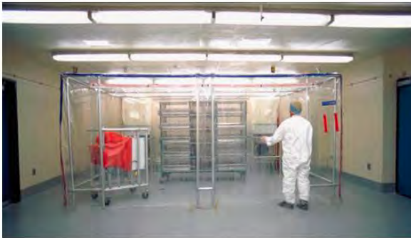
FIGURE 27.2 Negative pressure freestanding bioBUBBLE® enclosure. This unit is designed to be used for avian research requiring a primary containment system. Cages are located in the center of the enclosure and a bioBUBBLE® bedding disposal system is located in the front left corner of the enclosure. The disposal system is used for control of dust and allergens during cage waste disposal procedures. Two HEPA-filtered blower motors are present, one located in each of the back corners of the enclosure. Photo provided courtesy of bioBUBBLE®.
